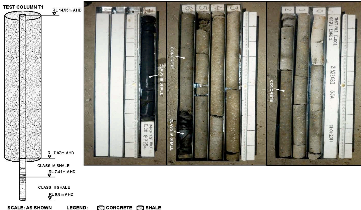
Figure 5. Coring test column T1
